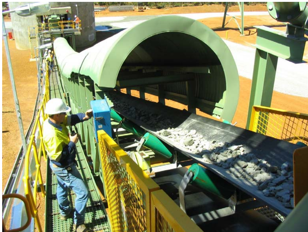
Figure 1. First Ore being conveyed from the coarse ore bin to the SAG mill
